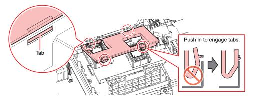
7 Remove the maintenance liquid absorber.
