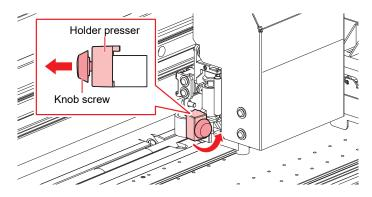
**5** Insert the cutter holder into the tool holder.
