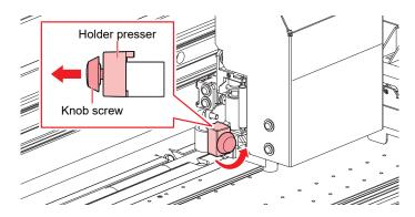
**5** Insert the pen holder or pen adapter into the tool holder.
