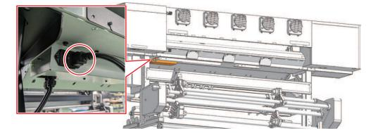
**2** Check to confirm that the power plug is connected to the power outlet.
