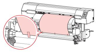
**23** Press O to wrap the media about one and a half turns around the paper core, then press the [ENTER] key.
