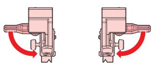
**A** Move the X cutter to the side and raise the lever to secure it.
