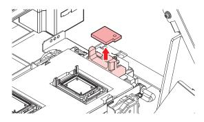
**Q** Wipe away any maintenance liquid from around the slider block.
