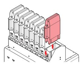
**2** Remove the ink absorber, and replace with a new one.
