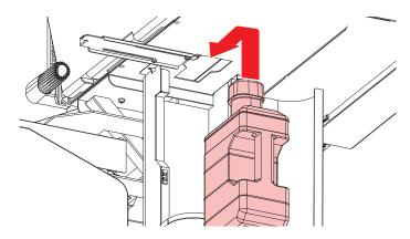
8 Return the stopper to its original position and close the waste ink tank cover.
