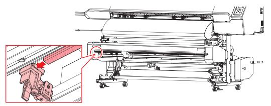
**2** Turn the screw and remove the cutter.
