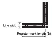
The recommended register mark length and line width are as shown below. The machine may fail to detect register marks that lie outside the recommended range.
