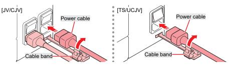
**5** Plug the power plug into the power outlet.
