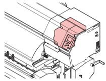
The UCJV is equipped with a UV-LED lamp, which cures the ink.
