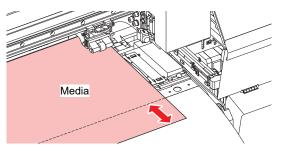
Lower the clamp lever to confirm that the spacing from the pinch roller is uniform.
