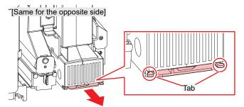
**5** If the glass holder is also replaced together, cut the tabs on the rear side.
