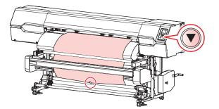
• If the media edge is straight, secure the left and right sides of the media. Pull the lower edge of the media evenly on both the left and right sides, check to confirm that it is free of sagging and creasing, then affix the tape.
