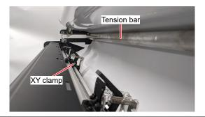
• If it is difficult to insert the media, the XY clamps should be individually unclamped, clamped, then unclamped again.
