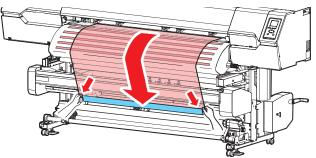
(3) Attach the media to the take-up unit, ensuring an even tension on both sides.
