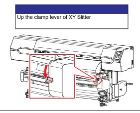
• The XY carriage can be moved by hand when the XY clamp lever is lowered.
