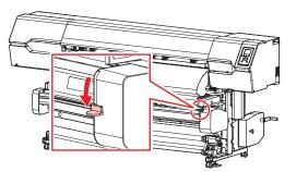
The XY carriage can be moved by hand when the XY clamp lever is lowered.
