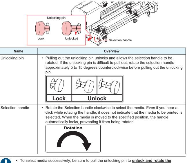
To select media successively, be sure to put the unlocking pin to <u>unlock and rotate the</u> selection handle. Attempting to rotate the handle without unlocking it may result in damage.
