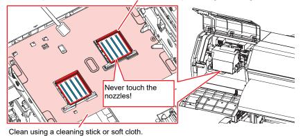
Clean the print head sides and all around the nozzle plate using a cleaning stick.
