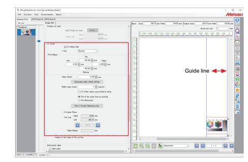
6 Select the [XY Slitter Edit] check box on the Image Edit tab.
