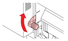
**2** Move the rear left roll holder to the roll setting position.
