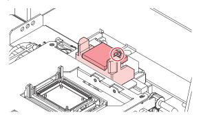
**9** Check to confirm that the absorber is not lifting or curved.
