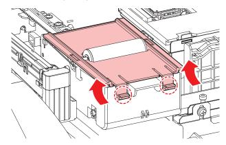
6 Remove the wiper together with the spindle.
