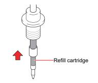
**3** Insert the spring into the refill cartridge.
