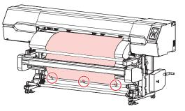
**10** Press **()** to wrap the media about one and a half turns around the paper core, then press the [ENTER] key.
