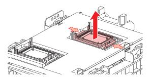
**5** [When using Sb ink and TP ink] Rinse the cap with the mesh side facing downward in a container filled with maintenance liquid. Remove, then wipe clean the resin part thoroughly.
