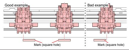
(motatt) Alter the XY clamp positions according to the RasterLink [Y Slit] setting.
