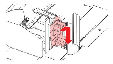
6 Attach the cap to the removed waste ink tank, and use tape to prevent leakage of waste ink.
