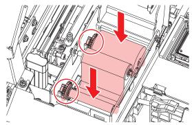
• If no cloth is wound around the spindle, wind the cloth around the spindle three times before mounting. If the cloth is mounted with no cloth wound around the spindle, the cloth may become detached from the wiper unit.
