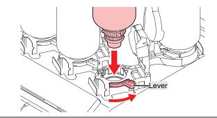
You may apply the maintenance liquid onto the O-ring of the ink bottle caps so that the ink bottle can be inserted easily. Use the appropriate maintenance liquid to suit the ink being used.
