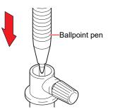
**3** Fix the pen nib by turning the knob screw in the direction indicated by the arrow in the picture.
