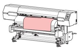
• Pressing the [FUNC2] key while the [Horizontal + V Cut] run screen is displayed creates a tape while simultaneously cutting the media. This can be used to tape the media to the paper core (only for self-adhesive media).
