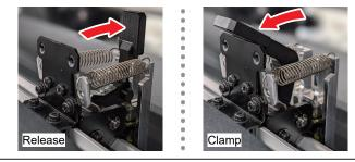
The XY clamps should be unclamped individually in locations where the media is not present. Note that they cannot be operated using the XY clamp lever if they have been individually unclamped.
