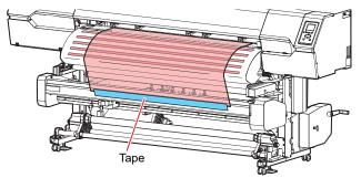
(2) Pull the media toward the take-up unit while spreading it out slightly evenly on both sides to prevent sagging.
