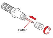
**3** Fix the cap by turning in the direction indicated by the arrow in the picture.
