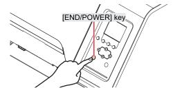
• Do not turn off the main power supply. Turning off the main power supply will disable the automatic maintenance function (including nozzle clogging prevention function and ink discharge channel cleaning function). This increases the risk of ejection failures (such as nozzle clogging or deflection).
