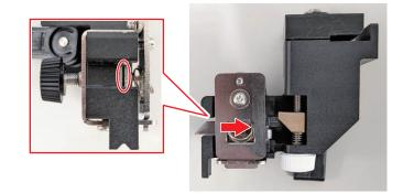
• If the blade does not stop, the blade is not positioned correctly. Reposition and insert the blade again.
