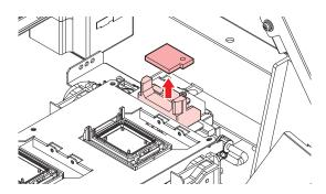
7 Wipe away any maintenance liquid from around the slider block.
