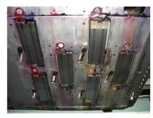
Soak the COTTON CIEGAL® in the maintenance cleaning liquid and wipe off the mark of the cap rubber attached on the nozzle surface from the rear side to the front side.
