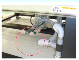
Due to heat from the exhaust port, it may be deformed.
