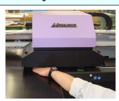
Do not put your hands into the gap between the carriage and the table with the power supply ON.
