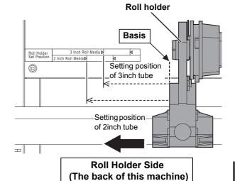
• Check the roll stopper is not caught between the roll stopper arm and this machine.
