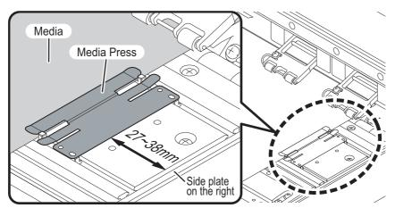
Media press position:27 to 38 mm from the side plate on the right. (For the variation of the inside diameter of media roll, it ranges as above.)
