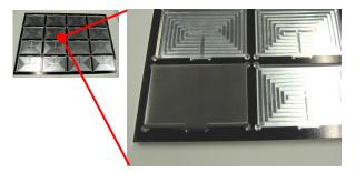
Prototype example for the card case jig (Aluminum is milling cut and the surface is painted in black)
